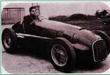
The post-war Tipo 125 1500-cc supercharged Grand Prix car being driven by Dino Ferrari. This was among the first cars built by the new Modena company.
